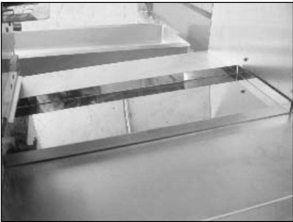
12. Install the oven crumb tray.
